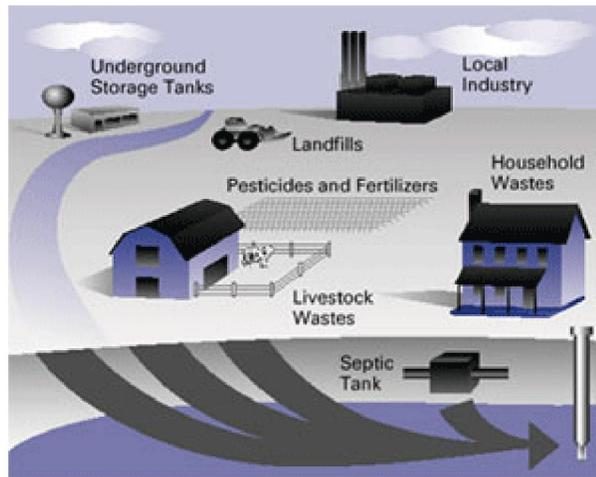
Septic tanks are designed to have a leach field around them, which is an area where wastewater flows out of the tank. This wastewater can also move into the ground water.
